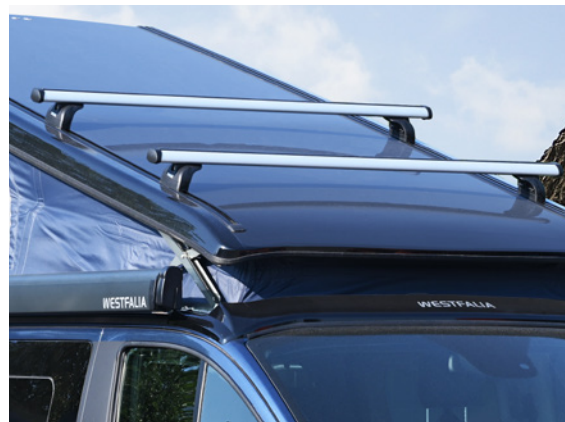
Thule roof rack for Nugget pop-up roof and Nugget Plus with pop-up roof (detailed view)
