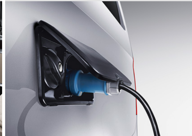
External connections for power and fresh water
