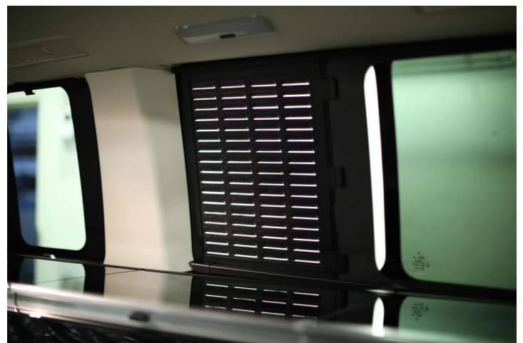
Air inlet for sliding window left
